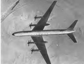
Flattened nose of the Tu 114 indicates that the aircraft has greater lift than wing carry as the Boeing 707 and the Douglas DC-8. However, the Tu 114's wing appears to have a higher aspect ratio which would make it more efficient for long range flight. These features are looked on with skepticism to reduce the spurious flow. Note change in taper ratio.
